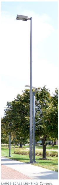
LARGE-SCALE LIGHTING Currently, West Broadway is lit by highway scale lighting that is much taller than pedestrian-scale lamp posts. This type of lighting may be appropriate in places along the corridor.
