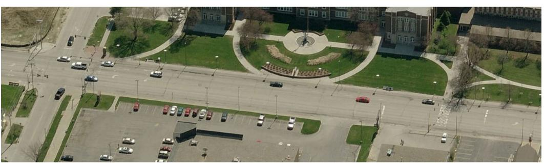
One of the few locations along the West Broadway Corridor where a median could be placed under the current roadway configurations, between Thomas Jefferson High School and Walgreens, where long stretches of the roadway are free from curb cuts
