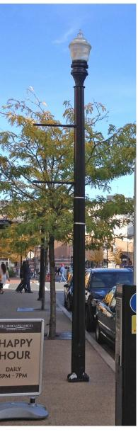
PEDESTRIAN-SCALE LAMP POST At nodes that connect to transit stations or urban spaces, pedestrian-scale lamp posts should be used at cross streets and along West Broadway.
